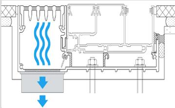
Single-level set down allows outstanding drainage and fast, easy installation.
