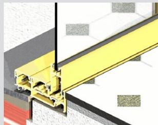
Semi and fully recessed sill options available to create seamless transition between internal and external. Semi recessed sill pictured above. Drains must be used with all fully recessed sill installations.
