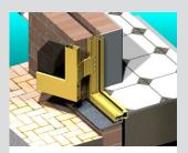
Fitting custom parliament hinges to French doors (80mm frame) allows panels to be opened back 180° to the wall lining when positioned correctly in building.
