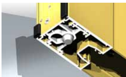
The stainless steel bolt tips are supported by extruded aluminium guides. This ensures the bolts fall in the right location and that they can withstand high wind loads when required.
