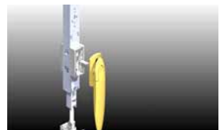
The bi-fold activator motor sits snugly in the frame and is positioned with nylon spacers again to ensure the bolts are in the right location in relation to head and sill.
