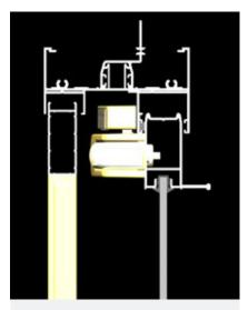
When used in the Series 471 Apartment door fitted with flydoors we recommend ANDO  $^{\rm TM}$  slimline as it clears the screen door.
