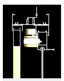
When used in the Series 47 I Apartment door the ANDO  $^{\text{TM}}$  slimline clears the screen door.
