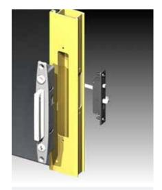
Mortice lock is securely fixed to window stile.
