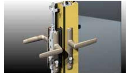
The dummy lock (keeper stile lock) can be operated from inside, turning the handle will retract the shoot bolts top and bottom.
