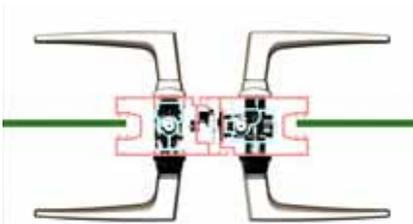
lever furniture is laid back to clear door stops. The furniture is available in a range of standard and special powder coated colours plus 316 grade stainless steel.
